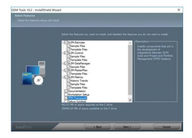
Note: When running setup in Maintenance mode, the check marks indicate already installed features and features that can be installed as a result of changes in your license agreement. If you uncheck any of the features on this screen, those features will be uninstalled during the update process.
