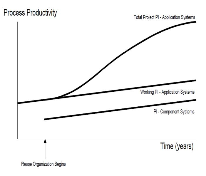
[Figure 1. The "working" productivity indexes of the application groups and the component groups rise slowly over the years, reflecting the slow growth in process productivity. Once component systems are available in some quantity for reuse the "total" productivity of the application groups grows exponentially until it reaches a new plateau, where reuse begins to near its limit.
