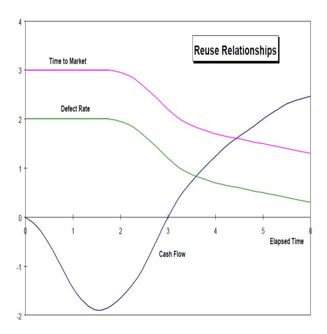
Figure 1. Investment is small during an initial period while a planning team is figuring out the reuse program. Costs grow when domain analysis and architectural work get under way and increase still more when component groups begin to function. After several years the gains from reusing component systems begin to offset the startup costs. As reusable components come into use, time to reach market declines. The defect rate follows a similar curve.
